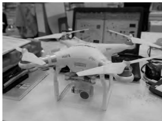
図-2 UAV実機(Phantom3)
