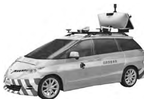
図 1 MMS (Mobile Mapping System)
