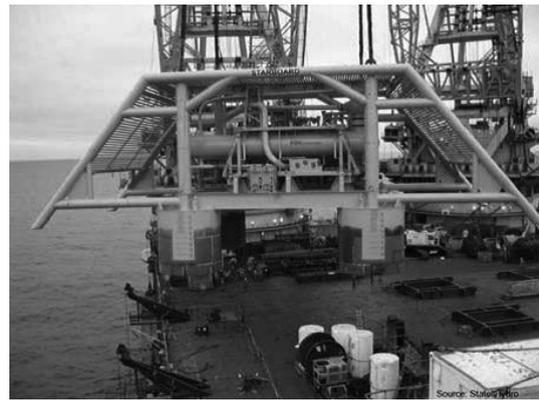
写真-4 Subsea Separation, Boosting and Injection system<sup>6)</sup>
