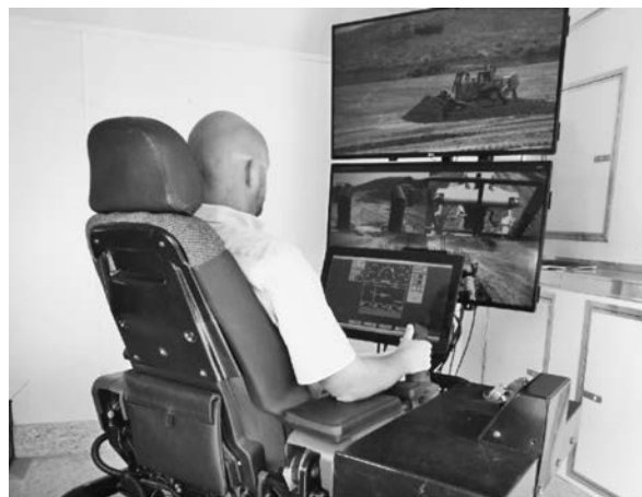
写真-2 Remote Operator Station の外観
