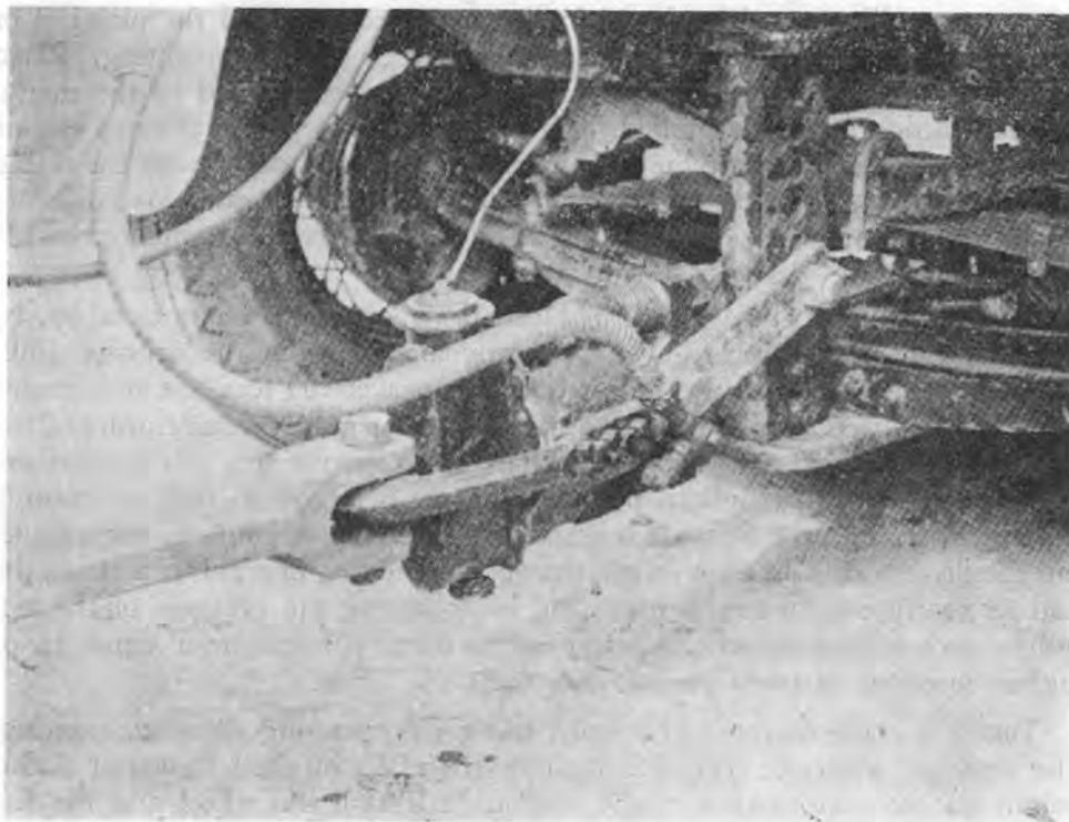
All of the pull exerted by the tractor is applied to the hydraulic draft unit.
