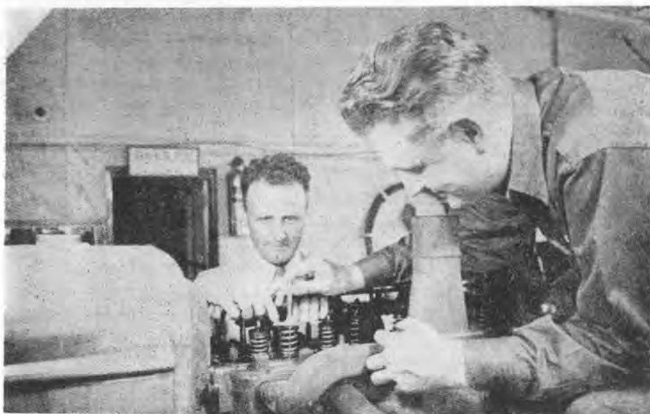
The valve lift is measured to check manufacturer's specifications.
