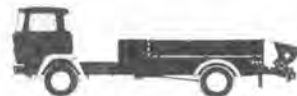
Auto Concrete Pumps: Models BPL 600 and BPL 800 arranged for subsequent mounting of a hydraulic luffing boom
