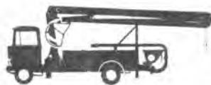
Auto Concrete Pumps: Models BPL 450 KVM 16 with 3-sectioned hydraulic luffing boom (16 m - 55 ft)
