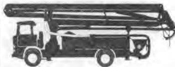
Auto Concrete Pumps: Models BPL 600 KVM 30 and BPL 800 KVM 30 with 3-sectioned hydraulic luffing boom (29 m - 95 ft)
