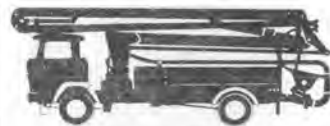
Auto Concrete Pumps: Models BPL 600 and BPL 800 KVM 25 with 3-sectioned hydraulic luffing boom (25 m - 82 ft)
