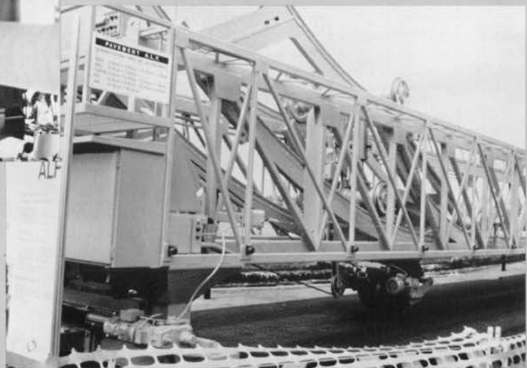
Accelerated Loading Facility ☞
