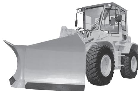
写真-4 KCM [AUTHENT] 55DV-2 除雪ドーザ
