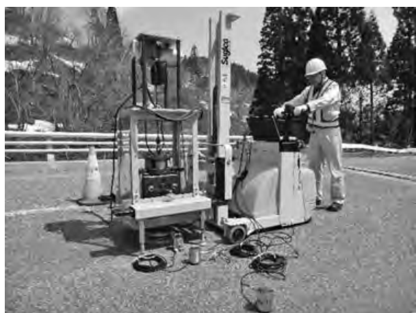
写真—2 衝撃加振装置 SIVE (Self-propelled Impact Vibration Equipment)
