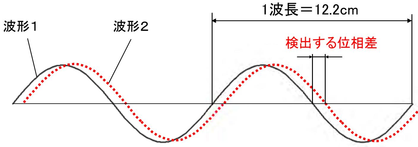
$$\text{位相差 } 1^\circ = \frac{\text{波長 } 12.2\text{cm}}{360^\circ} = 0.34\text{mm}$$
