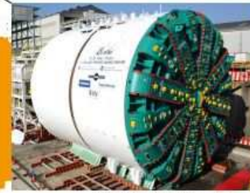
Φ17.45m泥土圧シールド [米国]
