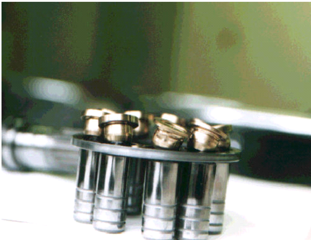
Appendix Figure 5 An example of abnormal wear on piston shoe
