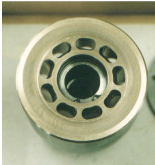
b) An acceptable example without any corrosion
