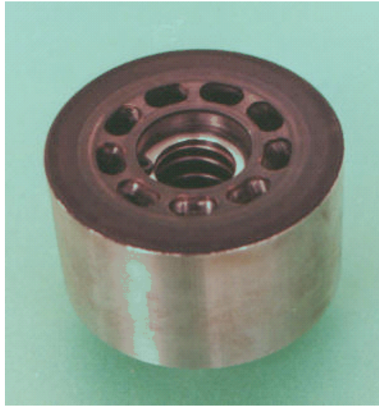
a) An unacceptable example due to corrosion thickness exceeding 1 \mu\text{m}
