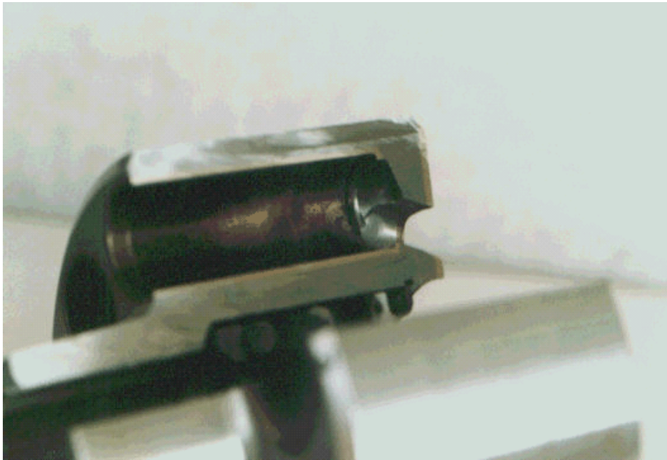
Appendix Figure 2 Unacceptable example with cavitation/erosion (arrow mark) inside cylinder (Cavitation/erosion occurring in the cylinder center may be disregarded if its diameter is less than 0.1mm.)
