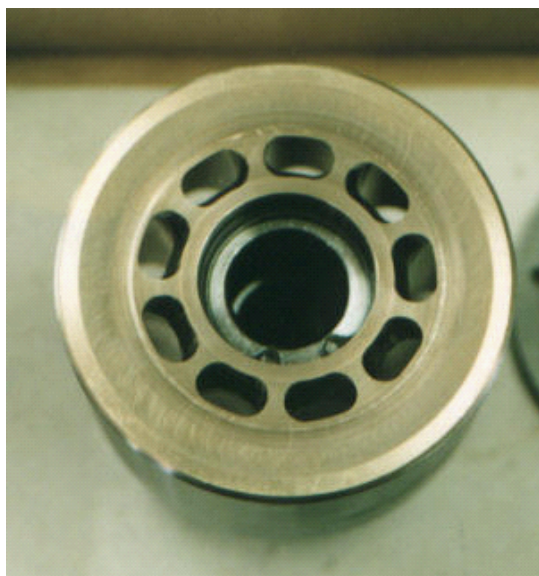
b) An acceptable example without any corrosion
