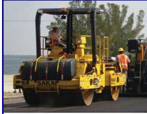
Sakai Intelligent Compaction equipped roller
