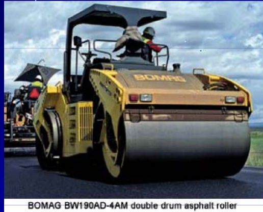
BOMAG BW190AD-4AM double drum asphalt roller
